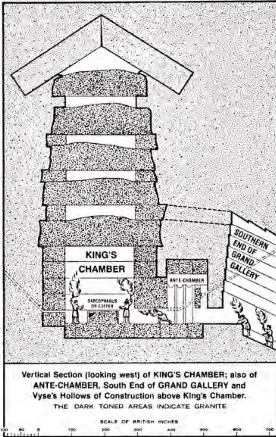
Vertical Section (looking west) of KING'S CHAMBER; also of ANTE-CHAMBER, South End of GRAND GALLERY and Vyse's Hollows of Construction above King's Chamber.
